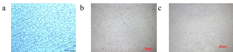
Fig. 1. Microstructure: a – continuous casting billet Ø 12.0 mm, obtained in EMM; b – rod Ø 5.0 mm after CRE; c - wire Ø 0.5 mm in annealed state, obtained with bar rolling with intermediate annealing and subsequent drawing
