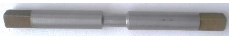
Fig. 2. Specimens made of steel 15Kh13N2 (AISI 414) for hot torsion tests in the Gleeble 3800 unit
