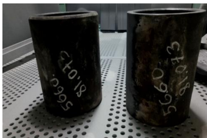
Fig. 1. Worn steel billet continuous casting machine rollers
