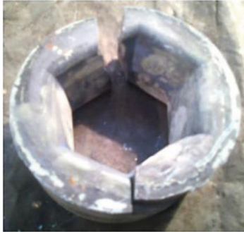
Fig.1. Destroyed carbide monolithic die by GOST 5426-76
