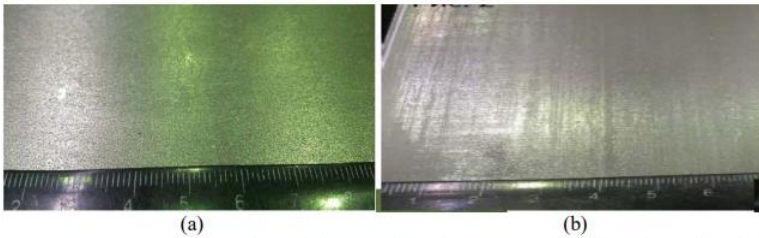
Fig. 1. Tempered strip surface of pilot run (a) and non-tempered strip surface of batch (b)
