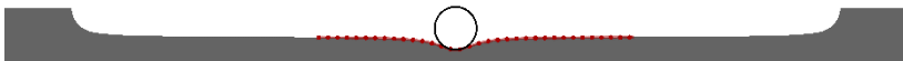
Fig. 1. The approximation of the neck profile with the help of Eq.1 based on FEM
