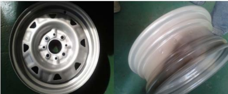
Fig. 2. Stamped wheel from pilot run of pickled temper-rolled strip of 07GBYu steel for the LADA automobile of JSC AvtoVAZ
