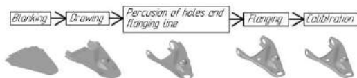
Fig. 1 – Process flow chart: Cold sheet stamping of front suspension arms for LADA LARGUS vehicles
