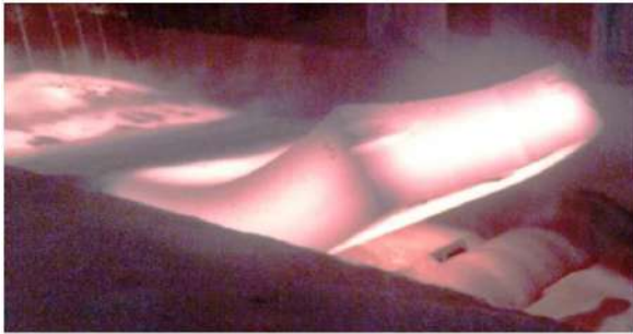
Fig.1 – Excessive upbending of the front end of the slab after stand 1 on mill 2000 of PJSC NLMK (for reference)
