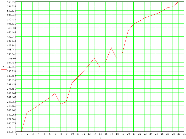
Fig.1 – Wire surface temperature change t_n in °C depending on fine drawing die number i (29 dies, including double dies)
